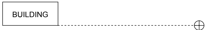
Figure 1: Semi-tangible reference point referenced to the corner of a tangible reference point.
