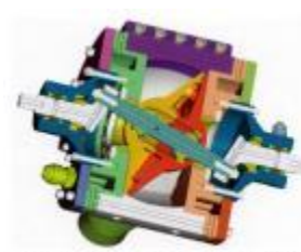
Figure 1. Single-disk nutating engine cross section.
